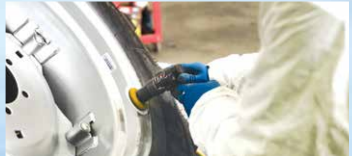
Wallenius Wilhelmsen team members preparing and inspecting wheels in preparation for painting.
