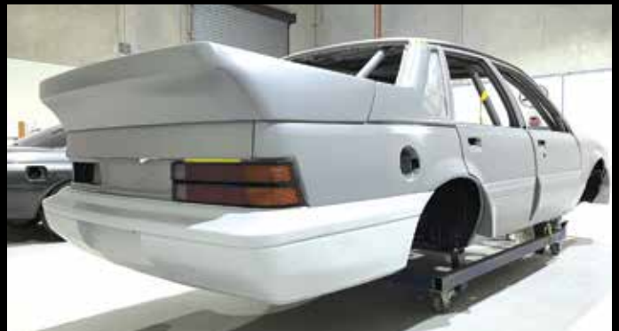
VL Walkinshaw in the trial fit stage before paint preparation.
