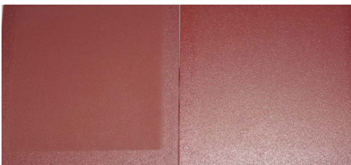
Gloss retention - Accelerated weathering QUVB 600h - Alesta® AP left/ Alesta® SD right
