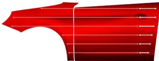
Apply second coat of the tinted clear to repair part and extend into adjacent panel (door). Ensure that you spray over the edge of the first tinted clear layer – staggered approach. Apply the second coat of the non-tinted clear to the widest area of the adjacent panel (door) and merge into the second coat of the tinted clear.
