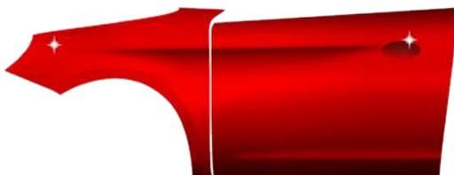
Another layer of the non-tinted clear over the entire repair area is recommended to simplify the subsequent polishing work. Slower product adjustments, longer flash-off and drying times should be considered. Dry the clear according to the technical data sheet. To improve the final topcoat appearance, this step can also be carried out after intermediate sanding with P1000.
