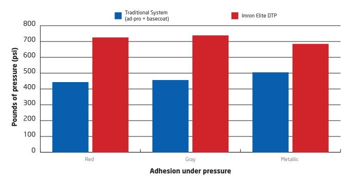
Three 20mm diameter dollies were glued on each test panel surface. Paint was cured 72+ hours before attaching dollies. Glue was allowed 72+ hours to dry. Results measured by PosiTest Pull-off Adhesion Tester.
