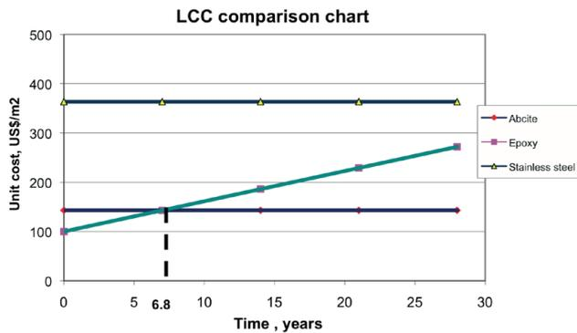
Figure 1. Lifecycle costs (LCC) – a comparison between stainless steel, epoxy and thermoplastic (Abcite). Image courtesy of Van Os-Duracoat, Belgium.
