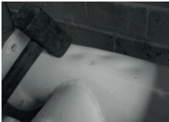
Figure 2. When hit with a hammer, the pipe will deform. The thermoplastic coating is able to adapt to the steel deformation, remaining undamaged and showing no failure or cracks. Image courtesy of Van Os-Duracoat, Belgium.
