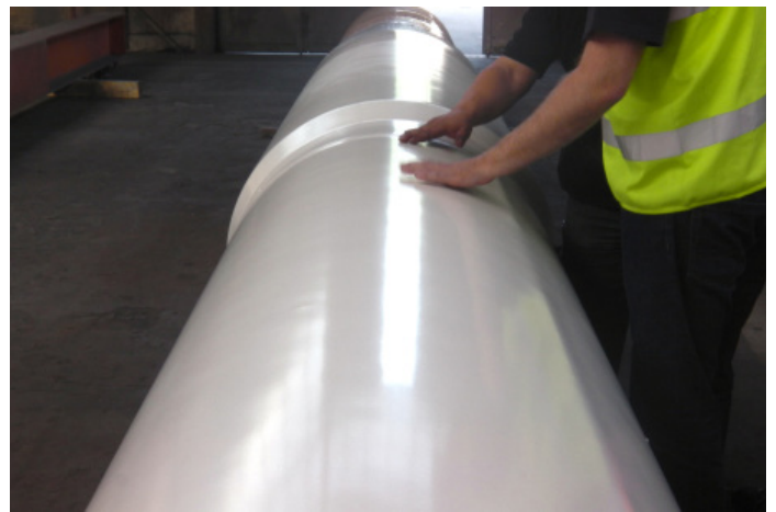
This buckle arrestor has been flame spray coated with Plascoat® PP10.
